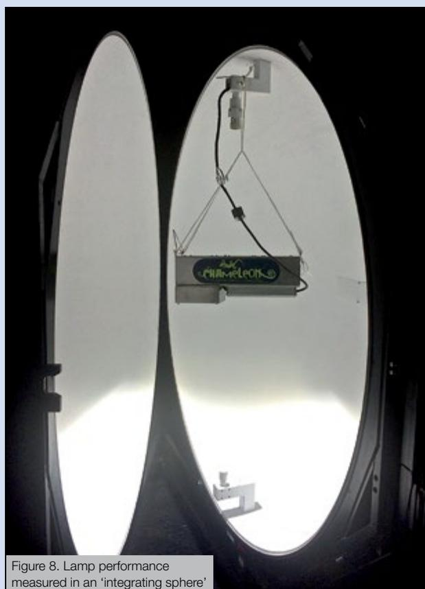
Figure 8. Lamp performance measured in an 'integrating sphere'
